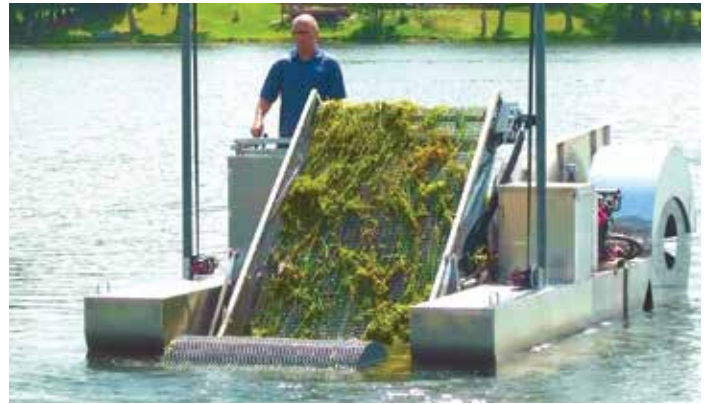
The "Eco-Harvester" provides an environmentally friendly and affordable method of invasive aquatic weed control. Photo courtesy of WeedersDigest.com
